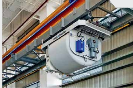
Concrete transportation system
