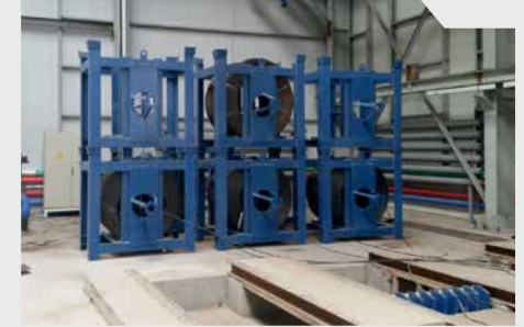
Store and decoil stressing wire
