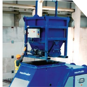
Concrete transport bucket
