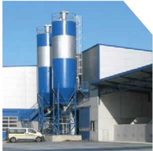
Concrete batching plant
